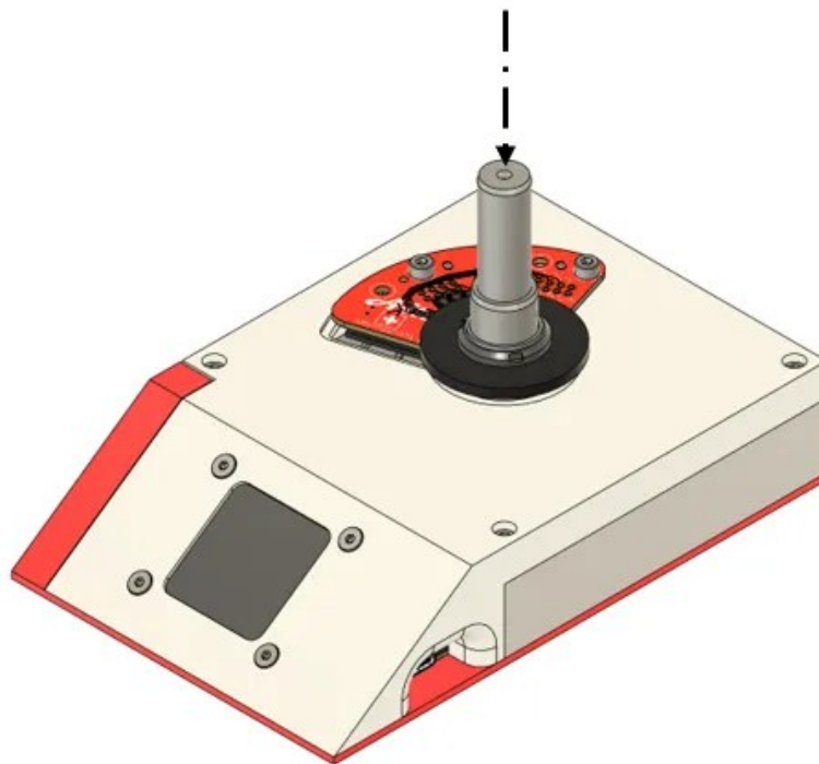
Figure 6: Assembly of the shaft with magnet
